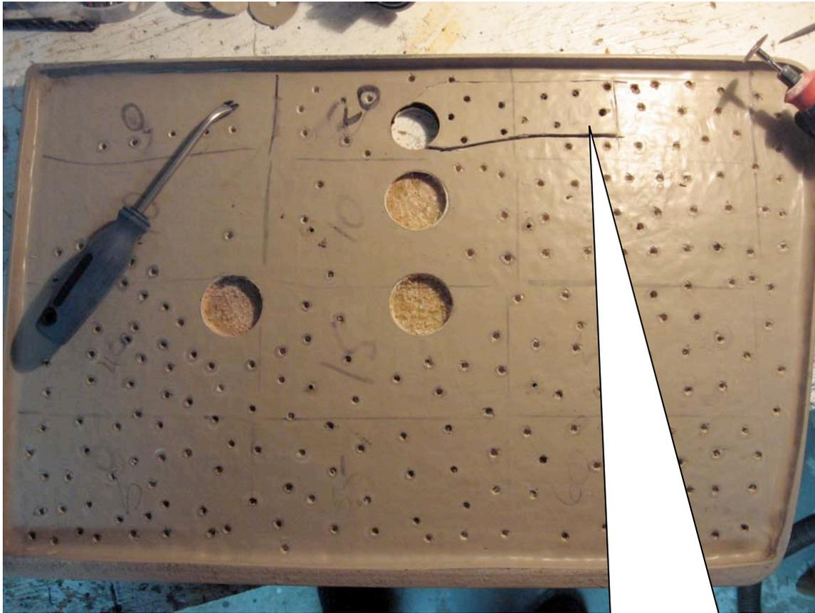
Drilling of these little vent holes produced blackened balsa in some locations, indicating the presence of rot. This section will be completely uncovered and the balsa removed. The whole hatch will be rebuilt once everything is dry.
