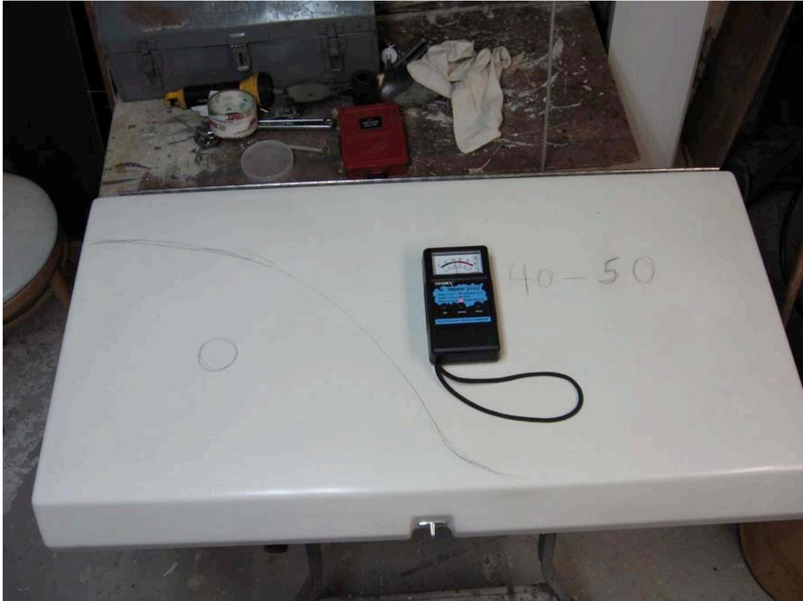
The same readings seen on the underside of the hatch cover. We can easily conclude that these moisture readings are the result of water entering via the piano hinge.
