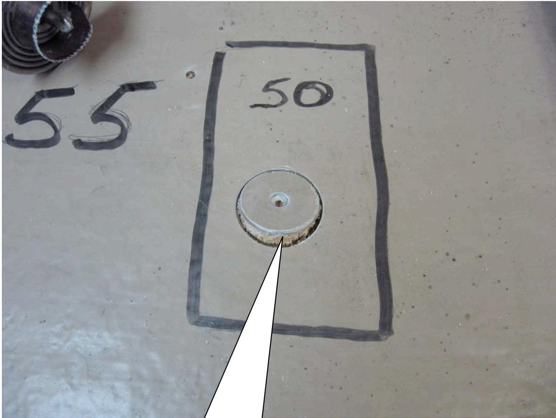
I immediately noticed moisture at this location, but neither delamination nor mould was apparent.
