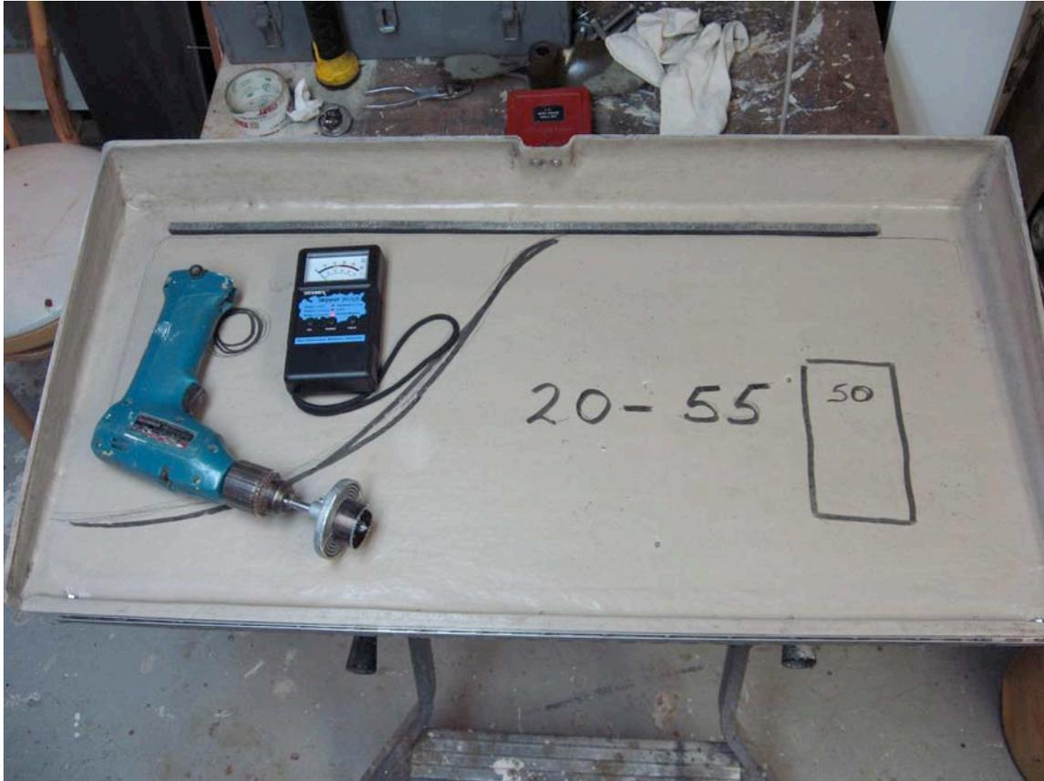
After drilling with the holesaw in the high-reading area, it was easy to remove the fibreglass disc within the cut.
