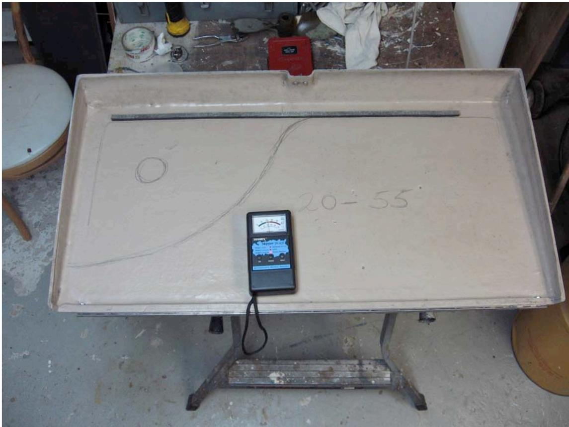
Getting more serious – Using a holesaw, I removed the top layer of fibreglass and bared the balsa within. I chose two locations for the holes, one where the reading was highest (50) and one with a reading of 0.
